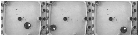
Fig. 8. The positions and orientations of the Magellan Pro robot in the arena during another experiment. On the left the robot is placed on the start position. In the middle the robot is placed on the goal position. On the right the robot is on the goal it finally found. Specified and found goals are perceptually identical, which is the reason for the outcome of this experiment
